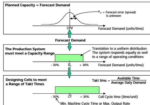
**Figure 5. Customer Demand and Takt Time, and Determination of Machine Cycle Time Range**
