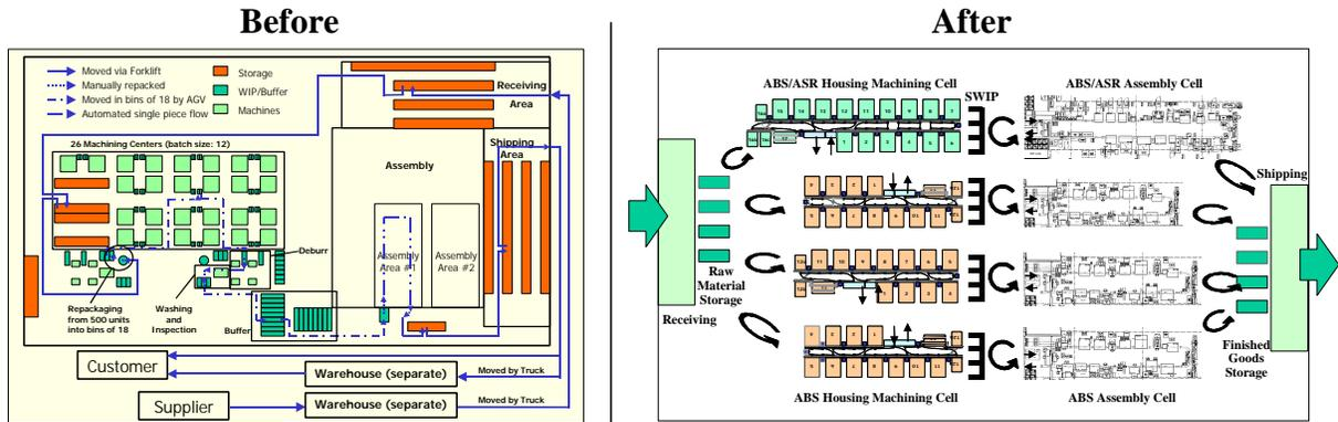
**Figure 7. Current System (left) vs. Newly Proposed Linked Cell Manufacturing System (right)**
