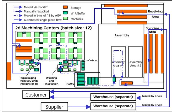
**Figure 1. Current Plant Layout and Material**
