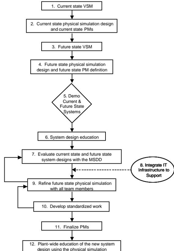
Figure 1. Flowchart of Change Process to Design and Implement a New Manufacturing System
