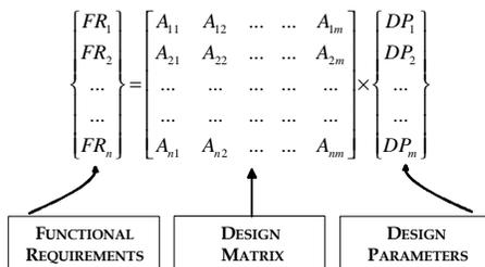
Figure 1. The Mapping process of Axiomatic Design
