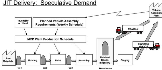
Figure 1. “JIT Warehouse” Due to Implementing Tools Not a Production System Design
