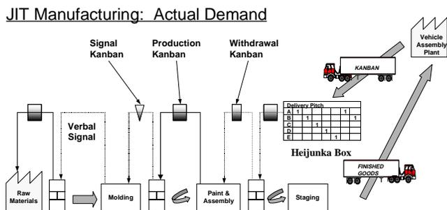
Figure 2. Information Flow and Equipment Re-design to Achieve Production System Design Objectives
